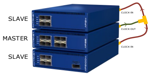
a) Multiple APG units synchronised locally
