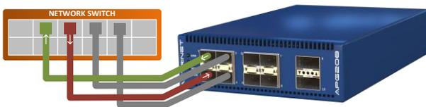
The first stream was configured to generate 1514 byte packets at 1% utilisation; with the second stream generating 64 byte packets at 95% utilisation.
