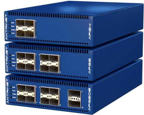
An intuitive Graphical Control Interface or TCL-scripted interface can be used to configure and control the packet generation, capture and analysis capabilities of the unit via a Linux or Windows PC, managing it locally over USB or remotely over Ethernet LAN.
