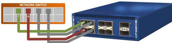
The first stream was configured to generate 1514 byte packets at 1% utilisation; with the second stream generating 64 byte packets at 95% utilisation.
